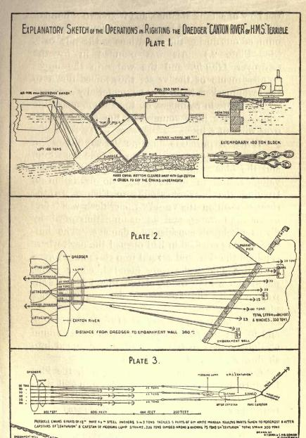
the bow of a tank steamer, and from two "lumps." These were filled and hove down at low water, and pumped out during the operations as the tide rose. (See Plate 2.) Air was pumped in by the destroyer *Handy*, and the water in the upper compartments of the vessel thus forced down to the level marked X on Plate 1, materially assisted.
